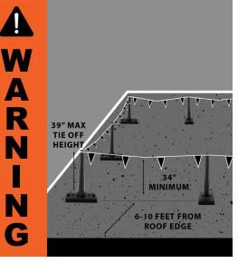
In accordance with OSHA 1926.502(f), and other regulations that may apply to warning line systems, this device shall be used by qualified personnel only. The warning line shall be rigged and supported in such a way that its lowest point (including sag) is no less than 34 inches from the walking/working surface and its highest point is no more than 39 inches from the walking/working surface.
